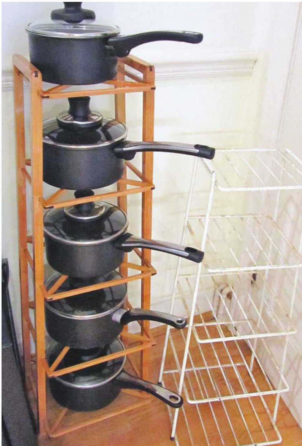
The finished stand, with the old wire-frame one alongside. Despite the new stand containing no metal except for 20 tiny panel pins, one in each corner of five shelves, it's coping with rough treatment
